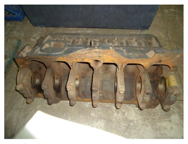
**DESCRIÇÃO DO BEM:** 01 (UM) BLOCO DE MOTOR OM366-LA MERCEDES BENZ SEM PISTÃO E SEM ANEL.
